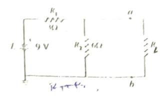
Also find out the condition for maximum power transfer in the circuit.
