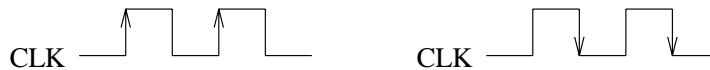
Figure 18: Clocks in timing diagrams for positive-edge triggered (left) and negative-edge triggered (right) devices.
