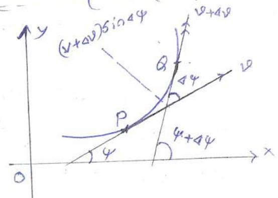
Let P be the position of the particle at time  $t$  & Q that in time  $t+dt$ .
