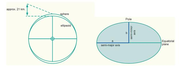
As can be seen from the dimensions of the Earth ellipsoid, the semi-major axis a and the semiminor axis b differ only by a bit more than 21 kilometres. A better impression on the Earth's dimensions may be achieved if we refer to a more "human scale". Considering a sphere of approximately 6 metre in diameter then the ellipsoid is derived by compressing the sphere at each pole by 1 cm only. This compression is rather small compared to the dimension of the semi-major axis a.
