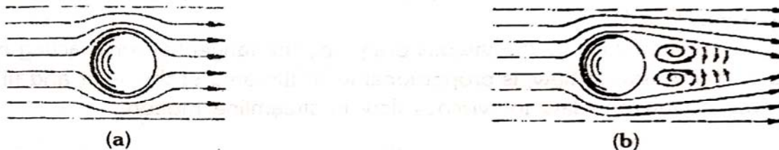
Fig 2: (a) Streamline flow causes no vortex behind the cylinder. (b) Vortex is formed behind the cylinder when water flows fast.
