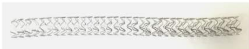
Fig. 2 Biodegradable polymer with Sirolimus coating on cobalt chromium stent.
